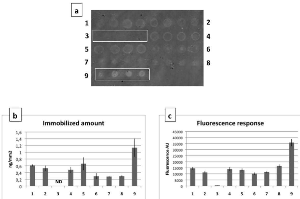
Figure 4-a: label free image of casein from bovine milk dissolved and spotted in PBS with 0.1% w/v SDS (1), PBS with 1% w/v SDS (2), PBS with 0.01% v/v Tween (3), borate pH 9 with 0.1% w/v SDS (4), borate pH 9 with 1% w/v SDS (5), borate pH 9 with 0.01% v/v Tween (6), saline-sodium citrate (SSC) buffer (7), phosphate/NaOH 50 mM pH 8.5 buffer (8) and NaOH 10 mM (9)
