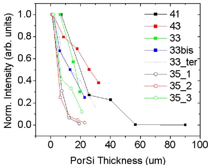
Figure 3 : decay of fluorescence through a porSi sample. Filled dataset represents samples spotted using high concentrated protein solution. Open symbols are for samples spotted with a more diluted solution. All porous silicon samples are fabricated from a (100) oriented silicon wafer.
